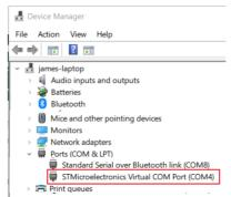
\* It will not work if 'STMicroelectronics Virtual COM Port' is not shown, and 3 things to check: a) Configuration Mode enabled? b)Driver installed? c) RFID device is connected to computer via USB cable?
